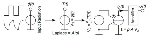
Fig. 4: Signal chain of the pyroelectrical system
