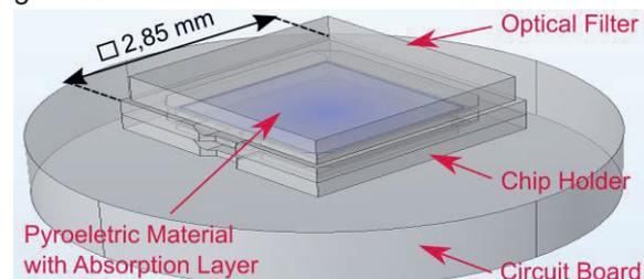
Fig. 2: FEM model of *LRM-244* with the thermal dominating parts. The surrounding air block is hidden.
