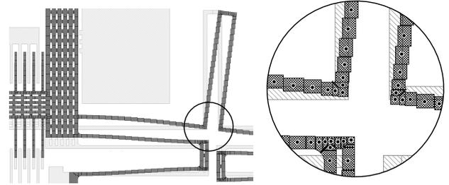
**Fig. 6:** Shifted tiles by FE-modal analysis displacement data.
