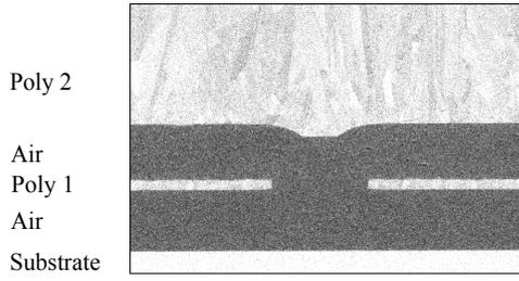
**Fig. 1:** REM picture of a cross section of a MEMS structure. The center of the picture shows the topography at the bottom side of the second layer (poly 2). This topography is caused by the structuring of the first layer (poly 1) during the fabrication process.
