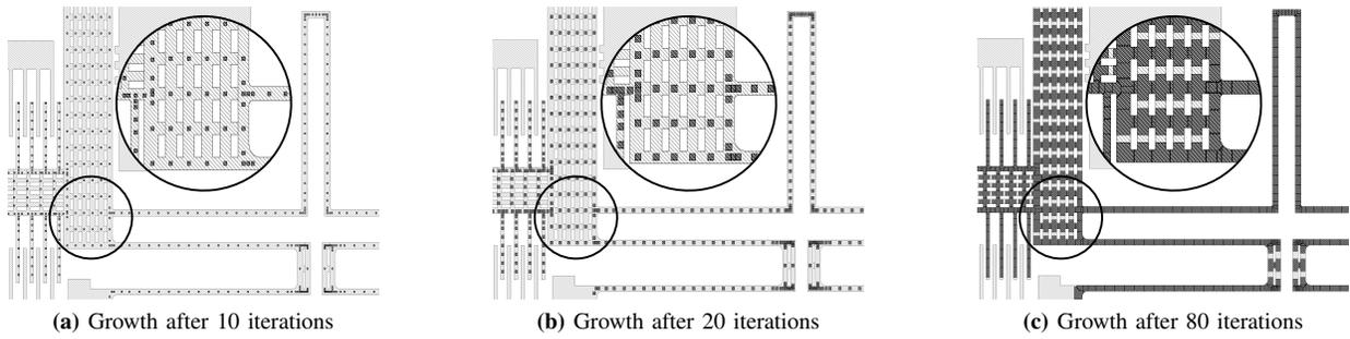
**Fig. 4:** Growth of the initial rectangles until they overlay the whole geometry.
