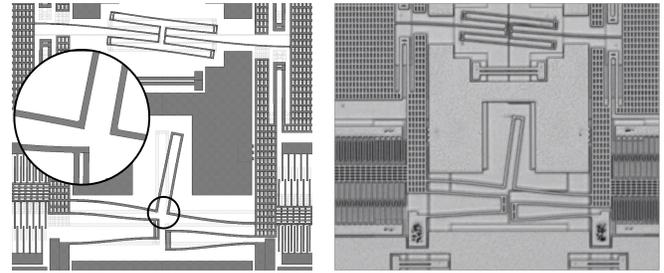
**Fig. 7:** The final deflected model for the electrostatic analysis compared to a microscopic picture of the deflected structure.
