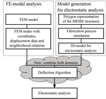
**Fig. 3:** Our approach for the quasi electrostatic analysis flow: combining the mechanical FE-modal analysis with the electrostatic model.
