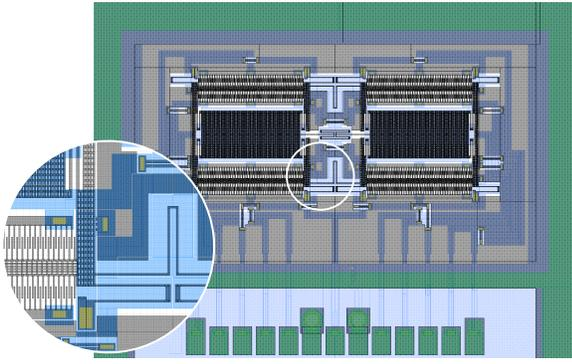
**Fig. 8:** Simple yaw rate sensor which is used for the demonstration.
