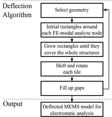
**Fig. 5:** The deflection algorithm flow.
