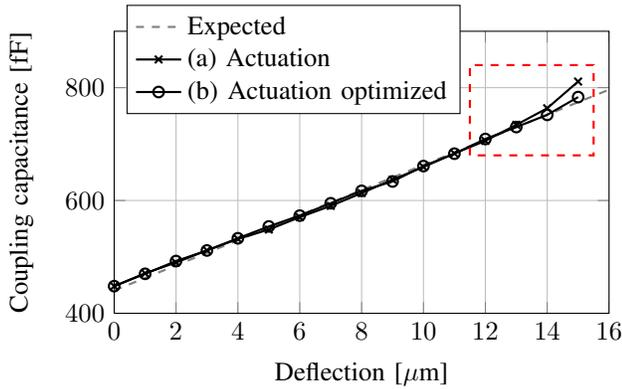
**Fig. 9:** Change of the coupling capacitances between the seismic mass and the drive combs in relation to the deflection: (a) before and (b) after optimization of the geometry.
