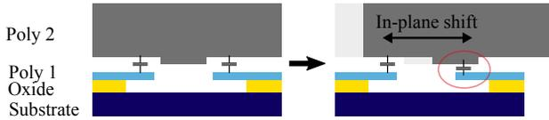
**Fig. 2:** Schematic cross section of a MEMS sensor structure. Poly 1 (blue): wires, Poly 2 (grey): mechanical structure. Left: The movable structure is in resting position. The coupling parasitic capacitances are symmetrical. Right: The movable structure is shifted. The parasitic coupling capacitance on the right side increases whereas the one on the left side stays constant.
