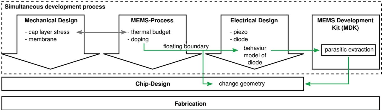
Fig. 2. Our design flow proposal for MEMS elements, featuring the simultaneous development of the mechanical design, the process technology and the electrical design. Due to the floating boundary conditions, the MEMS development kit (MDK) considers a parallel development of process technology and design. We highlight the influence of doping as floating process boundary to the electrical design and the chip-design in the figure.
