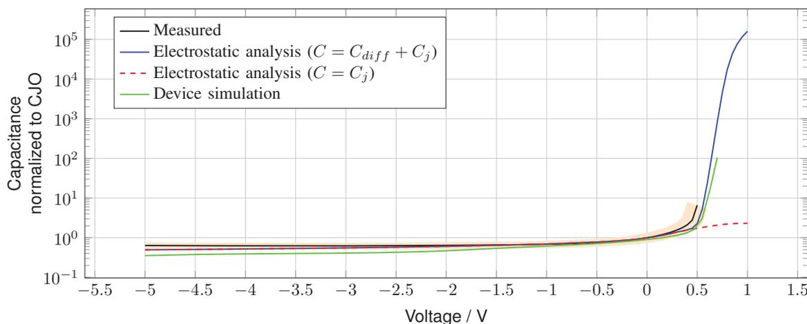
Fig. 4. Comparison of the measured and simulated junction capacitance of a pn-junction. The capacitance is normalized to the CJO (zero-bias junction capacitance) of the measured data. The orange band around the measured data visualize the possible statistical deviations of the measurements.  $C_j$  is the junction capacitance and  $C_{diff}$  is the diffusion capacitance.
