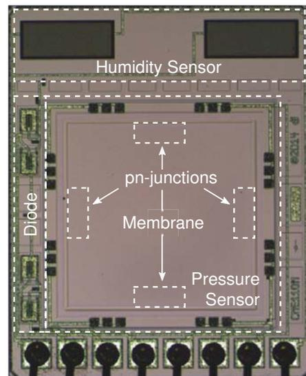
Fig. 1. Environmental sensor BME680 with pn-junctions [8], representing the piezo resistors of the Wheatstone-Bridge in the pressure sensor.
