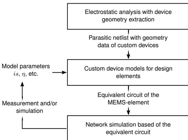
Fig. 3. Our electrostatic analysis flow for MEMS pressure sensors with active device elements.
