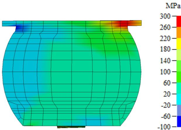
**Figure 9: Distribution of 1<sup>st</sup> principal stress within a corner solder ball of a TFBGA-104 package at the moment of first PCB deflection**
