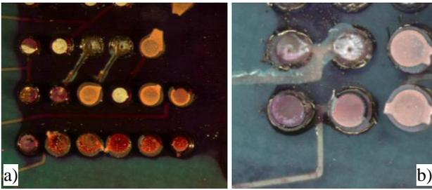
Figure 4: Dye and pry failure analysis of package types TFBGA-104 (a) and TFBGA-170 (b). Ultimate failure mode of both packages are lifted substrate pads.
