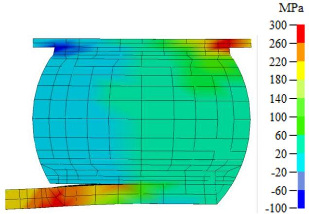
**Figure 10: Distribution of 1<sup>st</sup> principal stress at a corner solder ball of a VFBGA-90 package at the moment of first PCB deflection. The interconnection model includes a flaw between pad and solder due to the high stress orientation of the copper trace [17, 18].**
