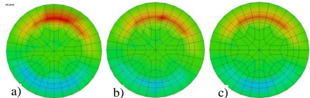
**Figure 11: Distribution of stress perpendicular to the substrate pad surface: a) TFBGA-104; b) TFBGA-170; c) VFBGA-90**
