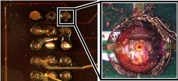
Figure 5: Failure analysis of package type VFBGA-90. The failure of the daisy chain is caused by a broken copper trace connection to a PCB pad.
