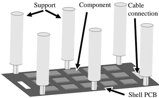
**Figure 7: Global simulation model of the JEDEC drop test setup including the PCB supports and the 15 components**
