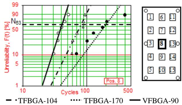
Figure 6: Weibull plots of the tested packages at component position #8
