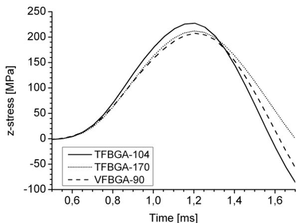
**Figure 12: Comparison of the maximum stress peaks in the substrate pads of the investigated packages**
