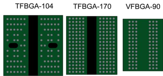
**Figure 3: Bottom view on the investigated package types TFBGA-104, TFBGA-170 and VFBGA-90**
