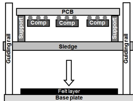
Figure 1: Schematic representation of the JEDEC drop test
