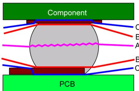
**Figure 2: Possible failure modes in a BGA solder ball.**
