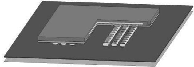
**Figure 8: FEM sub-model of a VFBGA-90 package including a cross-section through the component**
