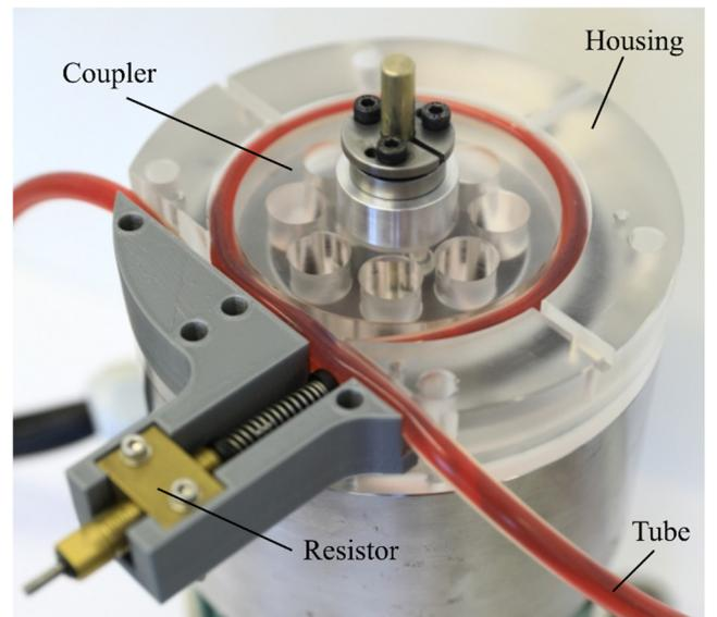
Fig. 4. Detailed view of the pump section of the experimental pump. A silicone tube is used in the experiments.
