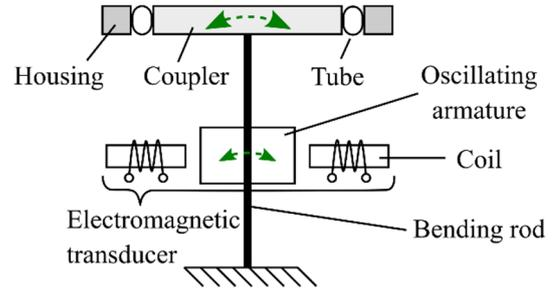
Fig. 3. Schematic illustration of the pump actuator in longitudinal section view (according to [5, 7, 8]). An oscillating armature motor generates the circulating eccentric oscillation (green arrows). The bending rod transmits the motion of the oscillating armature to the coupler.
