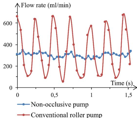
Fig. 6. Measured volume flow of the non-occlusive pump (continuous mode) in comparison to a conventional roller pump.
