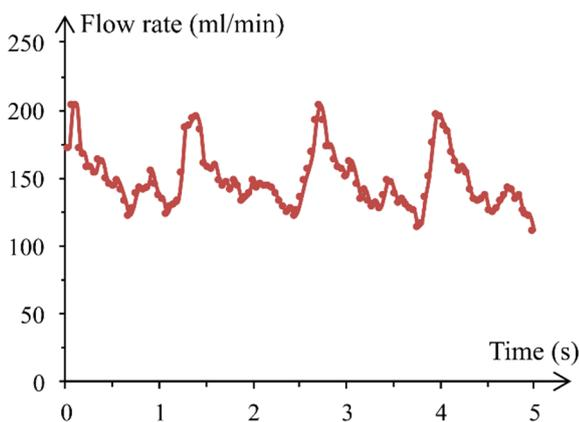
Fig. 8. Generated pulse shape with reference to the pulse shape of a second generation vessel in the human arterial network (according to [4]).
