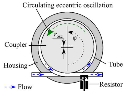
Fig. 1. Top view of the rotationally symmetrical pump section. The coupler performs a circulating eccentric oscillation with frequency  $f$ , oscillation amplitude  $r_{osc}$  and angle  $\varphi$  of oscillation.
