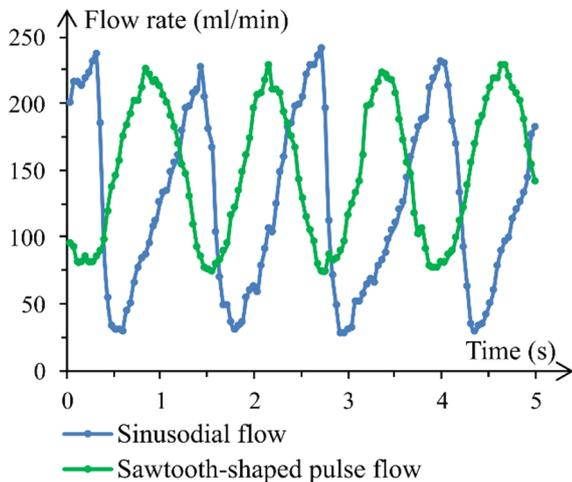
Fig. 7. Examples of generated volume flow pulse shapes. Multiple pulse forms can be realized with the non-occlusive pump by modulating the oscillation amplitude  $r_{osc}$ .
