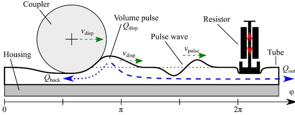
Fig. 2. Unrolled surface view of the pump section. The pumping principle of the non-occlusive peristaltic pump is based on a combination of volume displacement  $Q_{disp}$ , backflow  $Q_{back}$  and pulse wave propagation. The resistor decouples the volume flow at the pump outlet.
