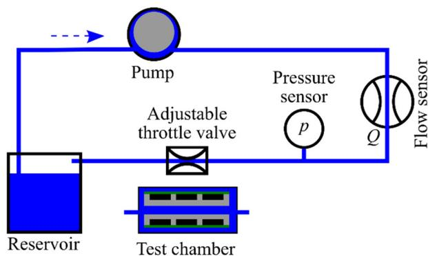
Fig. 5. Schematic illustration of the test circuit used for the experiments. The test chamber can be added for material characterization tests.
