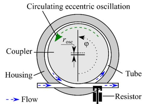
Fig. 1. Top view of the rotationally symmetrical pump section. The coupler performs a circulating eccentric oscillation with frequency  $f$ , oscillation amplitude  $r_{osc}$  and angle  $\phi$  of oscillation.
