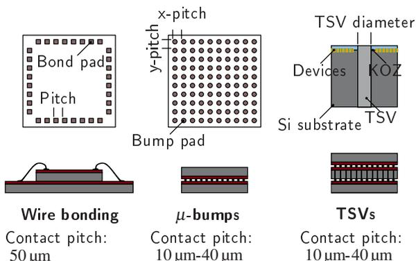
**Figure 2** The three most important package-level interconnect technologies: wire bonding,  $\mu$ -bumps and TSVs.
