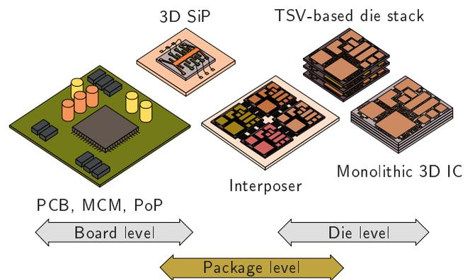
**Figure 1** Electronic systems can be subdivided into board-level, package-level and die-level integrated systems.
