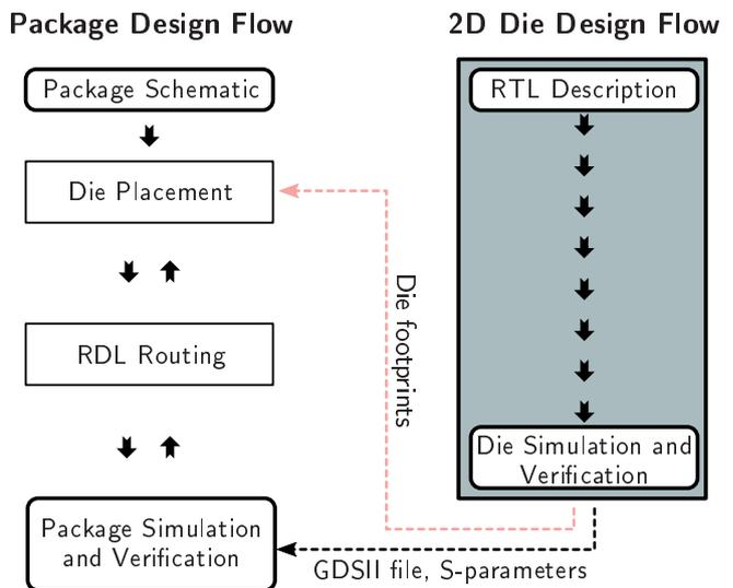
**Figure 4** Illustration of the *chip-driven design flow*. IC layout and package design are performed sequentially, allowing almost no interaction between the design processes. After 2D die design is finished, the die footprints are imported in the package layout tool to enable package-level die placement. Based on the die placement, the RDL routing is performed. GDSII files and parasitics can be included in package-level simulation and verification to enable accurate results.
