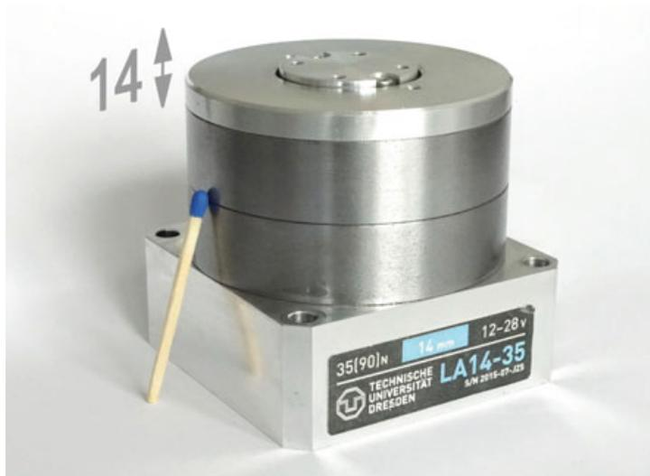
lateral stiffness decreases. At maximum mover deflection of  $\pm 7$  mm it is approx.  $0.1 \text{ N}/\mu\text{m}$ . Hence, flexure-guided actuators are suited for applications without or with moderate lateral forces, e.g. EDM or focusing and steering of optical beams.
