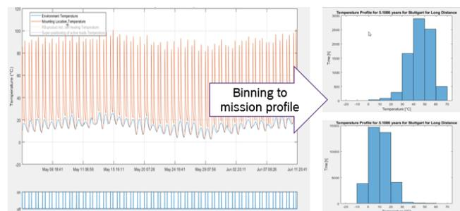
Fig. 4. Mission profiles for constant temperature and thermal cycling (on the right) are derived by binning from transient temperature profiles (on the left), in this case, for a commuter in Stuttgart.
