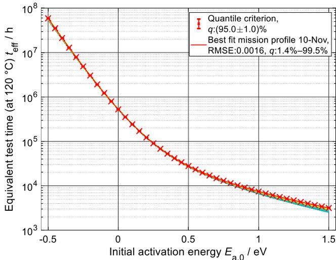
Fig. 7. Equivalent test times are derived for a failure mechanism that exhibits non-linear damage accumulation. Exemplarily, the mission profile of an engine compartment of a commuter driving in Stuttgart is evaluated with different purchase dates to select the best fitting date for the 95 % quantile criterion.
