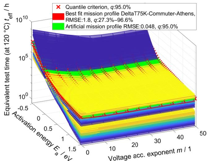
Fig. 5. Equivalent test times derived from multidimensional mission profiles of the interdependent stressors temperature and voltage. Color coding and raw data correspond to those in Fig. 2.
