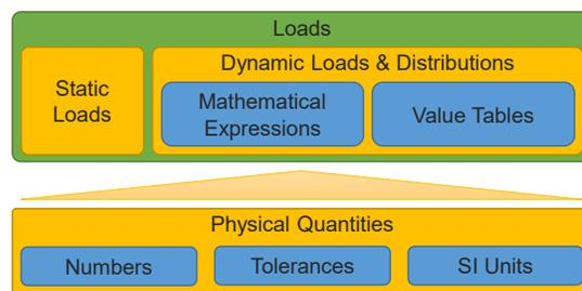
Fig. 12. Load definition using mathematical primitives in the electronic MPFo data format.
