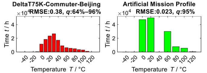
Fig. 3. a) Best fitting mission profile and b) numerically fitted artificial MP to represent the quantile criterion of Fig. 2 in order to facilitate the communication of this MP reliability requirement along the supply chain.
