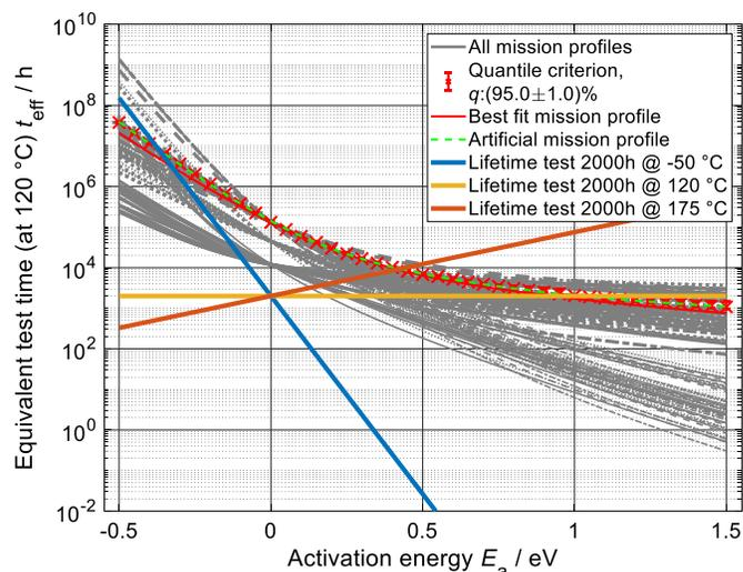
Fig. 10. All mission profiles from Fig. 2 are displayed in gray color and overlaid with the ETT representations of performed lifetime tests at different test temperatures. Since these lifetime tests have different behaviors, they cover different sections of the 95 % quantile criterion MP requirement on the activation energy axis.
