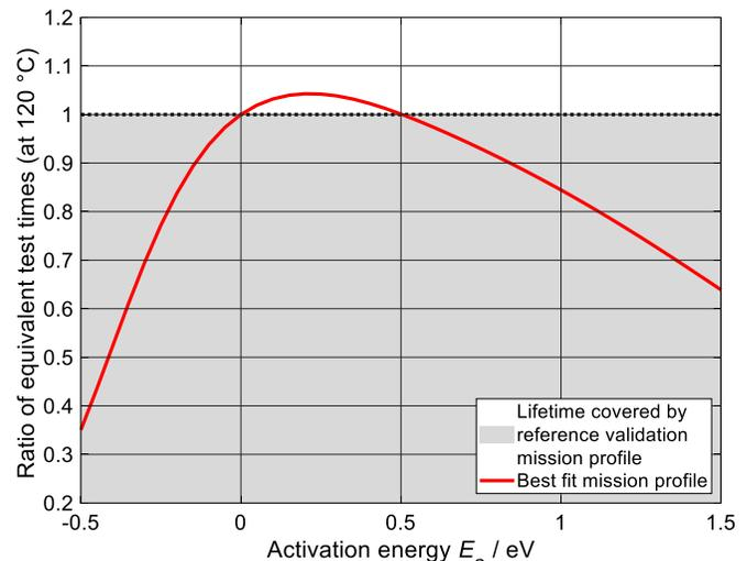
Fig. 11. The best fit mission profile from Fig. 10 is compared with the validation mission profile from Table I to deduce the degree of coverage.
