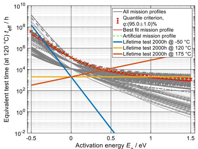
Fig. 10. All mission profiles from Fig. 2 are displayed in gray color and overlaid with the ETT representations of performed lifetime tests at different test temperatures. Since these lifetime tests have different behaviors, they cover different sections of the 95 % quantile criterion MP requirement on the activation energy axis.
