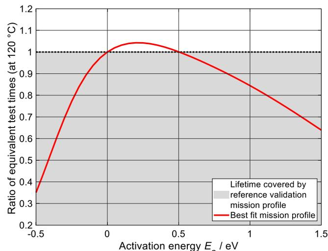
Fig. 11. The best fit mission profile from Fig. 10 is compared with the validation mission profile from Table I to deduce the degree of coverage.
