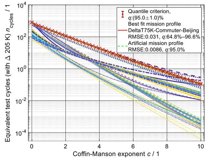
Fig. 8. Equivalent test times of the same 88 different automotive mission profiles from Fig. 2 are evaluated here for different acceleration parameters  $c$  of the Coffin-Manson model for temperature cycling. Color coding and raw data correspond to those in Fig. 2.
