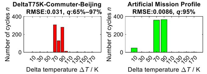
Fig. 9. a) Best fitting mission profile and b) numerically fitted artificial MP of the quantile criterion in Fig. 8.
