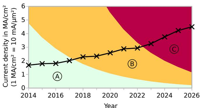
Figure 1. Expected evolution of required current density for driving four inverter gates for leading edge technologies according to ITRS roadmap [1]. As also shown, the maximum tolerable current density limits are shrinking due to smaller structure sizes. Region A / green: local EM issues, region B / yellow: all wires EM-affected, region C / red: no EM-solutions known yet.
