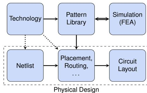
Figure 3. Layout synthesis using our proposed pattern verification method.
