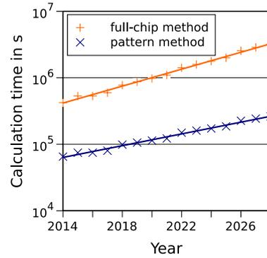
Figure 9. Comparison of estimated calculation times between full-chip analysis and pattern method for  $s = 1$  (one circuit verification per pattern library), calculated from technology parameters from [1].
