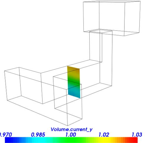
Figure 6. Verifying homogeneity of the current density at the cut surface between the two sub-models (3% maximum deviation here) ensures that distinct and combined simulations show matching results.
