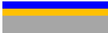
(c) Deposit photoresist
